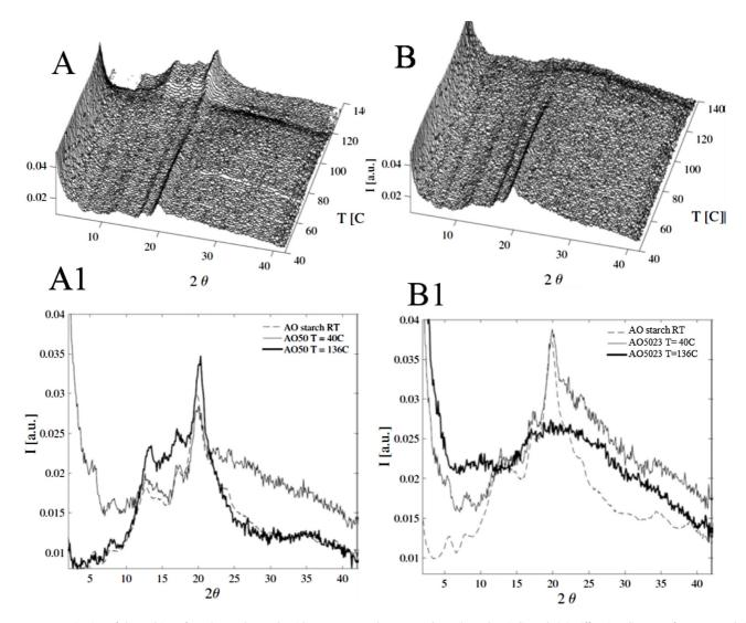
**Fig. 3.** X-ray monitoring of the melting of amylose-only starch with 50% water and 50% water/23% glycerol as indicated: (A) Diffraction diagram of AO50 recorded at 3 °C min<sup>-1</sup>, (A1) Overlay of AO50 diffraction diagram at T = 40 °C, T = 136 °C and T = 25 °C. (B) Diffraction diagram of AO5023 recorded at 3 °C min<sup>-1</sup>, (B1) Overlay of AO5023 diffraction diagram at T = 40 °C, T = 136 °C and T = 25 °C.
