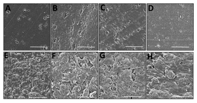
Fig. 7. SEM micrographs of cross-sectional and external surfaces of extruded starches. Cross sections: (A) A05 min (B) A010 min (C) A020 min (D) control. External surfaces (E) A05 min, (F) A010 min, (G) A020 min (H) control. Scale bars show 50  $\mu$ m.
