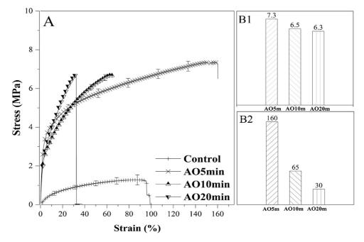
Fig. 5. Mechanical properties of extruded samples. (A) Stress and strain overlay of extruded samples with the control; (B1) Stress at break (MPa) and (B2) Elongation at break (%) of prototypes.
