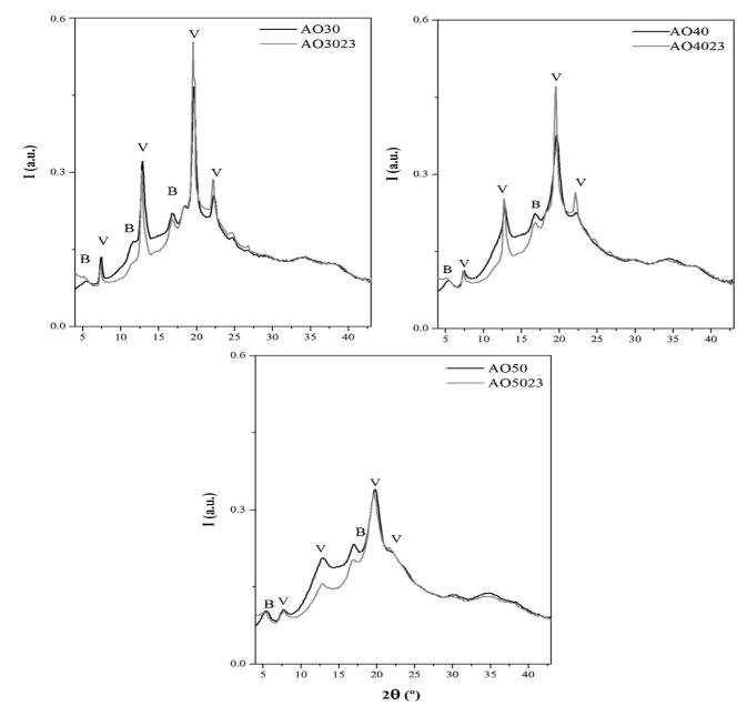
Fig. 4. Diffractograms of thermo-molded samples demonstrating the effect of different water and glycerol contents on crystal formation: (A) Overlay of AO30 and AO3023; (B) Overlay of AO40 and AO4023; C) Overlay of AO50 and AO5023.
