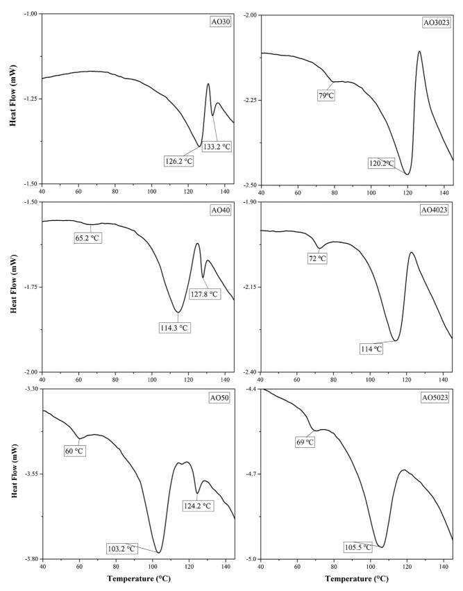
**Fig. 2.** DSC thermograms showing the effect of glycerol on the thermal phase transition behavior of AO as a function of water  $\pm$  glycerol content. Water-only systems: AO30, AO40 and AO50; water plus glycerol systems: AO3023, AO4023 and AO5023, as described in the text.
