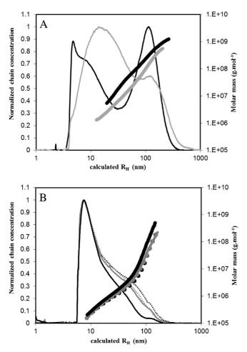
**Fig. 1.**  $R_H$  (thin lines) and molar mass distributions (bold lines) of native and extruded samples. A) control(black) and extruded control starch(grey), B)AO(black, solid line) and extruded AO5 min (black dotted line), AO10 min (grey solid line), AO20 min (grey, dotted line) starches.
