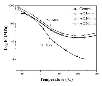
**Fig. 6.** Storage moduli of all extrudate samples measured by DMA showing the effect of amylose on the increase in the stored energy compared to control starch (The E' value shown is calculated at  $T = 25 \degree$ C).
