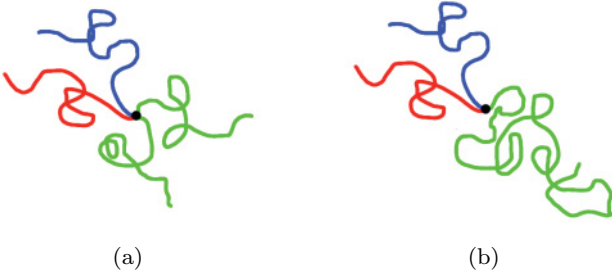
FIG. 1. (Color online) The topology of the miktoarm star copolymers investigated here. (a) An ABC_2 star. (b) The corresponding ABC star with matching composition. Both structures correspond to x = 2 .
