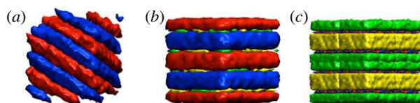
Figure 4. Lamellar structures found at the boundaries of the investigated phase diagram. (a)  $[\text{LAM}_3]$  structure found at  $x = 0.28$  with  $a_{ij} = 36$ . (b)  $[\text{LAM}_{\text{CD-in-AB}}]$  at  $x = 0.28$  with  $a_{ij} = 80$ . (c)  $[\text{LAM}_{\text{AB-in-CD}}]$  at  $x = 14$  with  $a_{ij} = 80$ . (a, b) show single box views, (c) shows  $2 \times 2 \times 2$  boxes.
