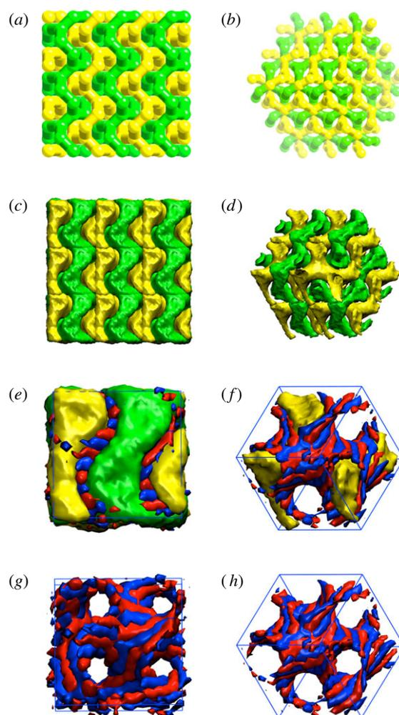
Figure 6. Alternating gyroid with hyperbolic lamellar interface [ $G_A$ ]. Left column show views along the [100] direction and right column along [111]. (a,b) Crystallographic models of two intertwin srs-nets. (c,d) Simulation snapshots of  $3 \times 3 \times 3$  boxes matching (a,b). (e)–(h) Single box views illustrating the AB hyperbolic lamellae membrane separating the two nets.
