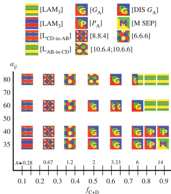
Figure 3. Phase diagram of a blend of ABC and ABD 3-miktoarm star terpolymers as a function of composition and interaction strength. The  $x$  parameter is indicated in the figure. Note that at some points in the phase diagram, two different phases were stabilized several times. These are indicated by half-sized icons.
