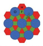
**Fig. 14** Schematic picture of the star-polyphile molecular arrangement in the 12.6.4 tiling found for the star-polyphile hexagonal mesophases. The dimensions of the green fluorocarbon domains compared with the molecular dimensions requires some interdigitation of fluorocarbon chains.
