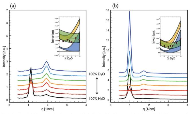
**Fig. 6** Experimental SANS scattering data for a series of (a)  $B-O_7-H_{16}-F_{10}$  with 10% water, and (b)  $B-O_7-H_{14}-F_8$  with 25% water samples measured at 35 °C with of varying  $H_2O/D_2O$  mixing ratios. Inset: Comparison between experimental and theoretical Invariant as describe in Figure caption 11.
