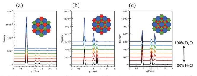
**Fig. 12** Simulated SANS scattering patterns for  $B-O_7-H_{16}-F_{10}$  star-polyphile samples containing 25% water assuming (a) an underlying 6.6.6-tiling, (b) an underlying 12.6.4-tiling, with the hydrocarbon chains filling the hexagons and fluorocarbon chains filling the quadrangles, and (c) an underlying 12.6.4-tiling, with the fluorocarbon chains filling the hexagons and the hydrocarbon chains filling the quadrangles.
