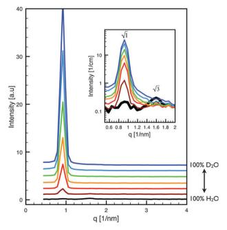
**Fig. 4** SANS scattering data for a series of samples with neutron contrast variation of  $B-O_7-(H_{16})_2$  with 25% water of varying  $H_2O/D_2O$  mixing ratios. (The scattering curves are shifted by an arbitrary factor for clarity.) Inset: magnified view of the peaks plotted with a logarithmic intensity scale.
