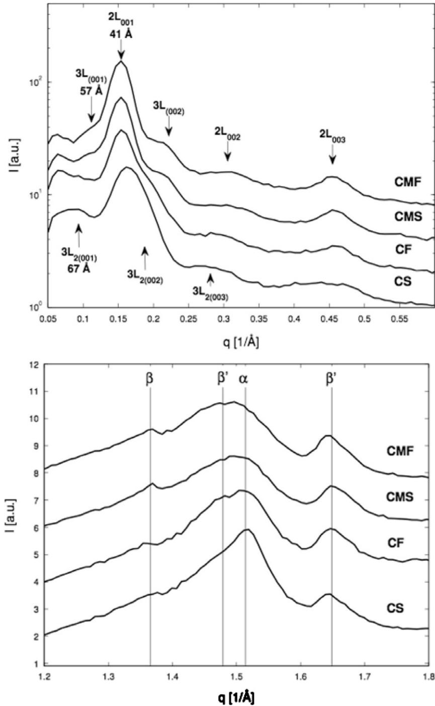
**Fig. 4.** SAXS (Top) and WAXS (Bottom) spectra from cream at 5 °C subject to different temperature treatments. CS: slow cooled cream, CF: fast cooled cream, CMS: slow cooled and matured cream and CMF: fast cooled and matured cream. Vertical lines indicate the positions of the characteristic peaks from the polymorphs forms:  $\alpha$ : 4.15 Å,  $\beta'$ : 3.81 Å, 4.2 Å,  $\beta$ : 4.6 Å (Lopez et al., 2005).
