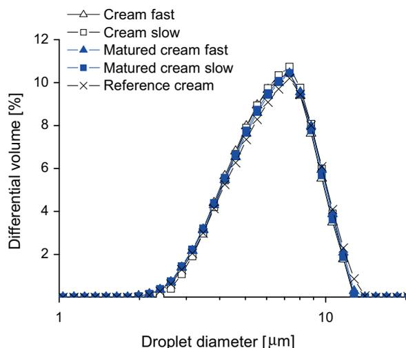
**Fig. 1.** Size distribution of milk fat globules obtained from light scattering measurements of cream. The cream samples were cooled from 65 to 10 °C either fast, 7.5 °C/min or slow 0.4 °C/min. Two samples were stored at 5 °C/min for 48 h after fast and slow cooling, respectively, while one was stored at fluctuating temperatures (3 h at 5 °C, 3 h at 20 °C, 8 cycles of 1 h at 20 °C and 1 h at 5 °C). Furthermore, a reference cream was analysed.
